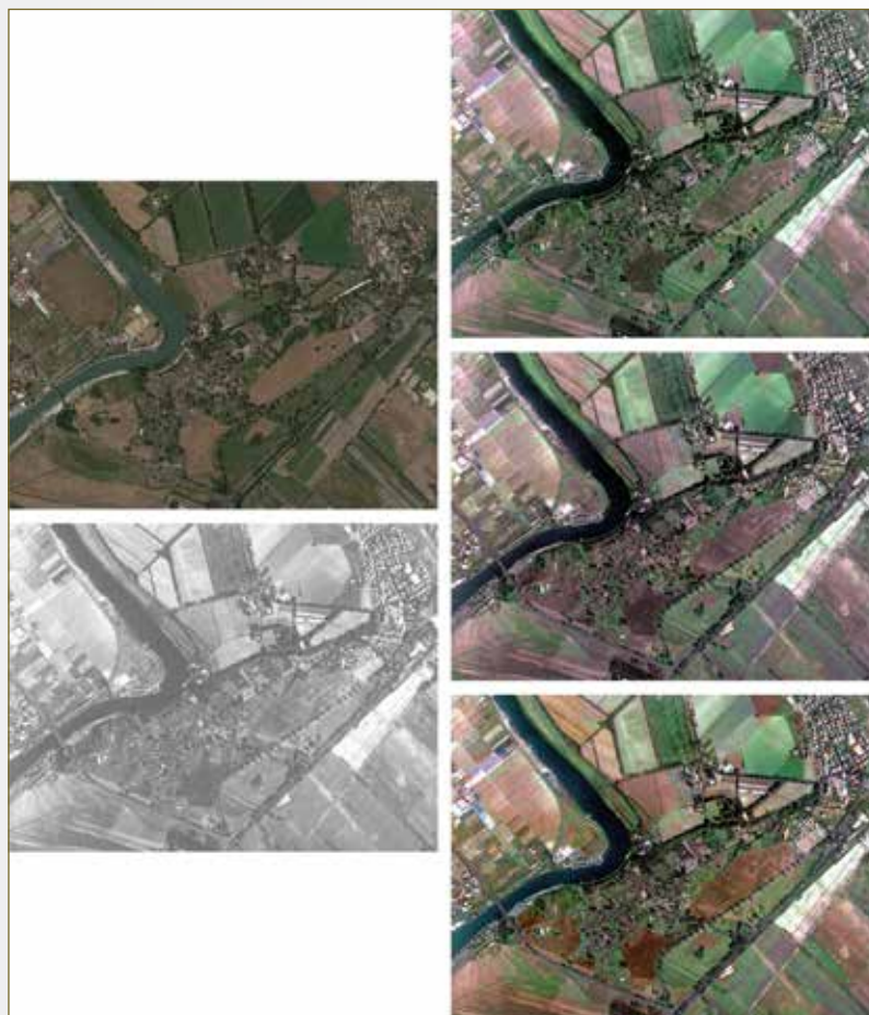
Fig. 1 - Example of pan-sharpening between a satellite image and an historical panchromatic photograph (top and bottom left). In the column to the right, three different algorithms, respectively (from top to bottom) Brovey, IHS and PCA.
